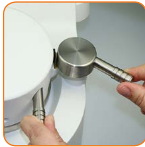
After heating time has elapsed, swivel pressure chamber over the model and close locking handle.
