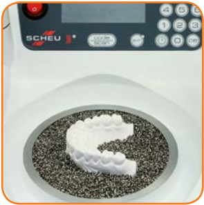
Place model on the platform or embed it into pellets and fix material with the locking ring.
