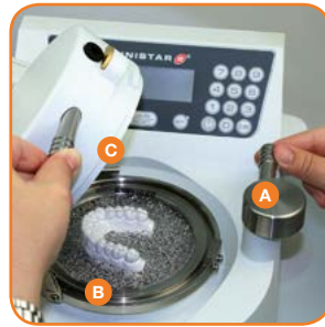
After cooling time has elapsed, open pressure chamber: A open locking handle B push clamping ring to the left C open pressure chamber
